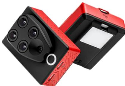
Fig. 2. Parrot Sequoia camera (the imaging and sunshine sensors are shown).
