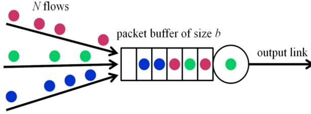
Fig. 1. The model of the queuing system.
