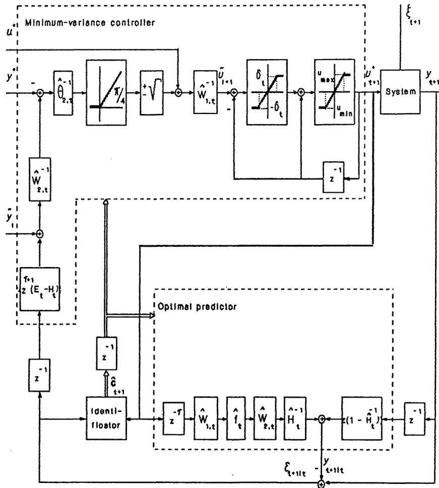
Fig. 2. The diagram of self-tuning minimum-variance control system.
