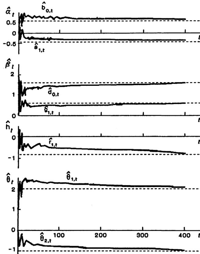
**Fig. 3.** The convergence of current parameter estimates for the system (45) in the self-tuning control process.
