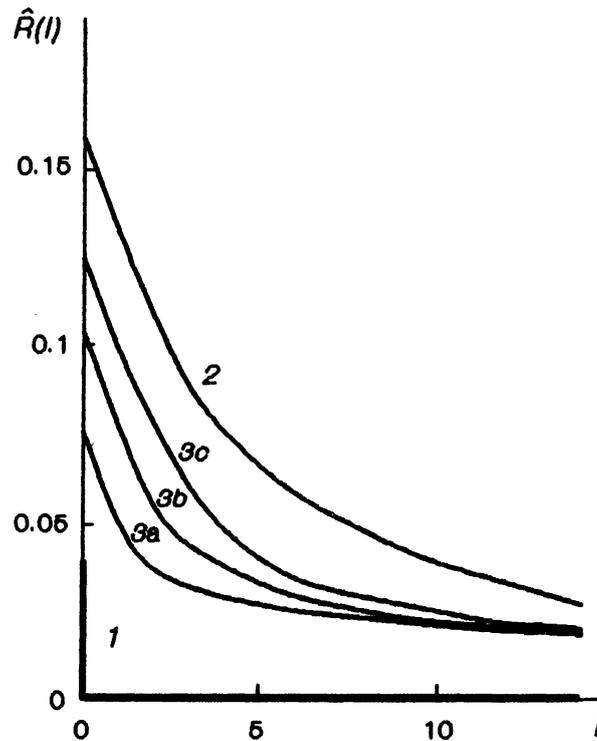
**Fig. 4.** The autocovariance function estimates for the system (45): 1 – for the white noise, 2 – for the disturbances at the output, 3 – for the control error: a – control with genuine system parameters without restrictions (46), b – self-tuning control without restrictions (46), c – self-tuning control with restrictions (46).
