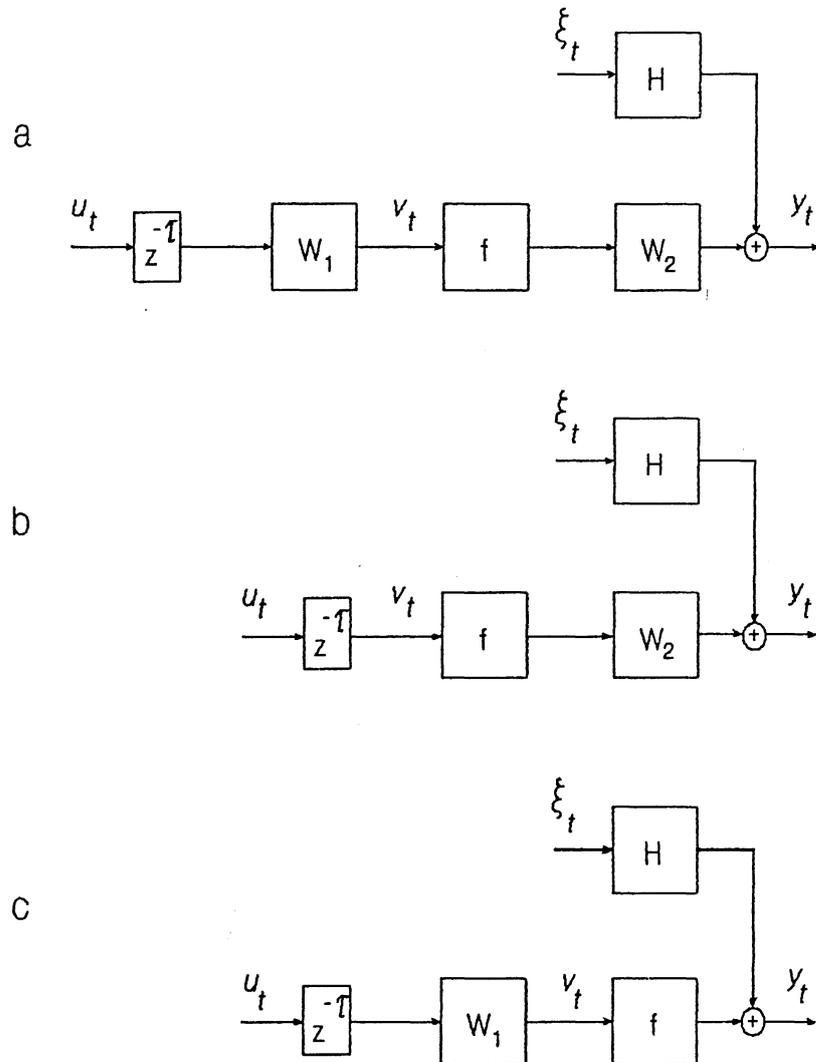
**Fig. 1.** Stochastic extremal systems of Wiener-Hammerstein (a), Hammerstein (b), and Wiener (c) types.
