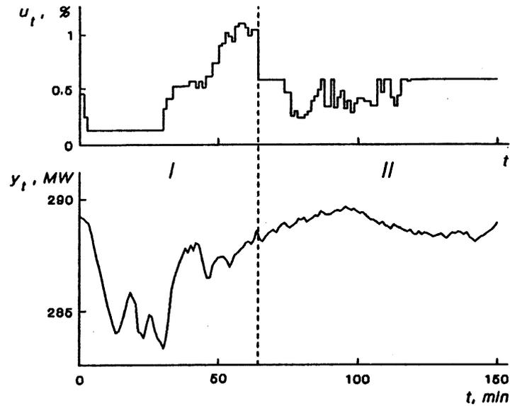
**Fig. 6.** The results of a numerical experiment on self-tuning control of fuel combustion process.
